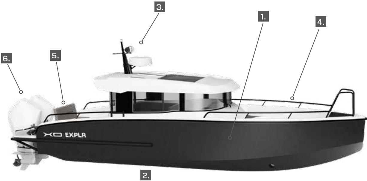
1. Long and narrow waterline with deep-v hull
