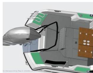
**RAILING ON AFT DECK WITH TOWING POLE**
