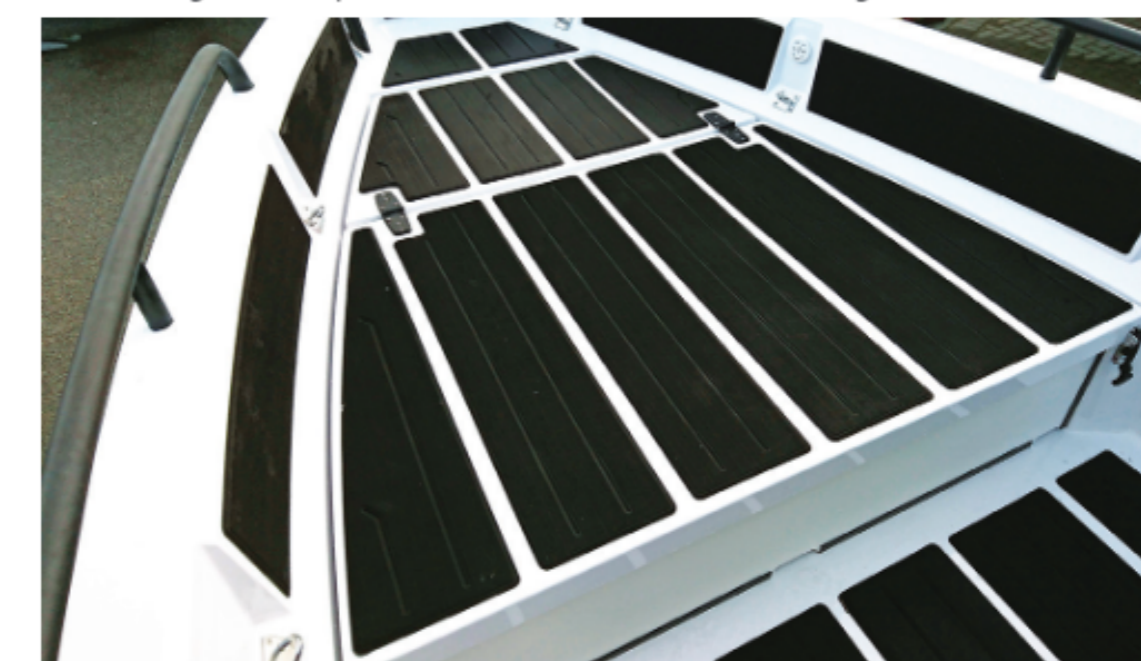
The bow locker's removable back panel allows longer items to be stowed.
